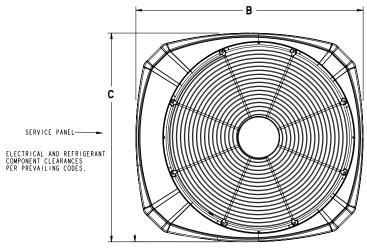
TOP DISCHARGE AREA SHOULD BE UNRESTRICTED FOR AT LEAST 1524 (5 FEET) ABOVE UNIT. UNIT SHOULD BE PLACED SO ROOF RUN-OFF WATER DOES NOT POUR DIRECTLY ON UNIT, AND SHOULD BE AT LEAST 305 (12") FROM WALL AND ALL SURROUNDING SHRUBBERY ON TWO SIDES. OTHER TWO SIDES UNRESTRICTED.
