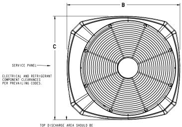
TOP DISCHARGE AREA SHOULD BE UNRESTRICTED FOR AT LEAST 1524 (5 FEET) ABOVE UNIT. UNIT SHOULD BE PLACED SO ROOF RUN-OFF WATER DOES NOT POUR DIRECTLY ON UNIT, AND SHOULD BE AT LEAST 305 (12") FROM WALL AN ALL SURROUNDING SHRUBBERY ON TWO SIDES. OTHER TWO SIDES UNRESTRICTED.
