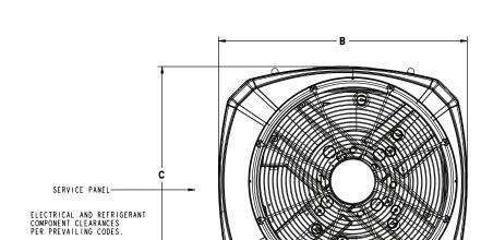
TOP DISCHARGE AREA SHOULD BE UNRESTRICTED FOR AT LEAST 1524 (5 FEET) ABOVE UNIT. UNIT SHOULD BE PLACED SO ROOF RUN-OFF WATER DOES NOT POUR DIRECTLY ON UNIT. AND SHOULD BE AT LEAST 305 (12") FROM WALL AND ALL SURROUNDING SHUBBERT ON TWO SIDES. OTHER TWO SIDES UNRESTRICTED.
