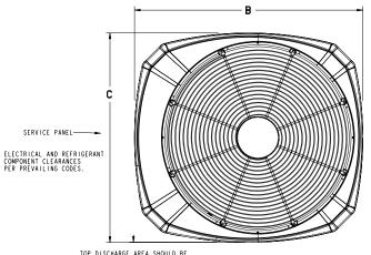
TOP DISCHARGE AREA SHOULD BE UNRESTRICTED FOR AT LEAST 1524 (5 FEET) ABOVE UNIT. UNIT SHOULD BE PLACED SO ROOF RUN-OFF WATER DOES NOT POUR DIRECTLY ON UNIT, AND SHOULD BE AT LEAST 305 (12") FROM WALL AND ALL SURROUNDING SKRUBBERY ON TWO SIDES. OTHER TWO SIDES UNRESTRICTED.
