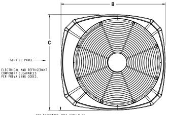
TOP DISCHARGE AREA SHOULD BE UNRESTRICTED FOR AT LEAST 1524 (5 FEET) ABOVE UNIT. UNIT SHOULD BE PLACED SO ROOF RUN-OFF WATER DOES NOT POUR DIRECTLY ON UNIT, AND SHOULD BE AT LEAST 305 (12") FROM WALL AND ALL SURROUNDING SHUMBBERY ON TWO SIDES. OTHER TWO SIDES UNRESTRICTED.
