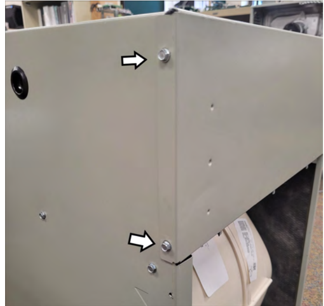
Figure 8. Bottom cross member panel screw location left side
