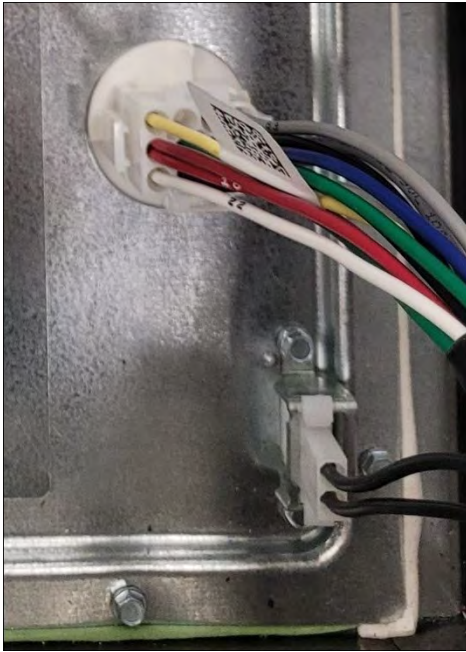
Figure 41. Line voltage interlock harness
