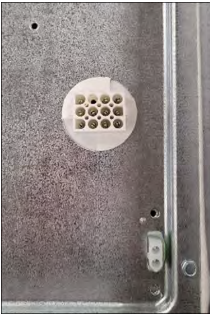
Figure 24. Reinsert blower connector
