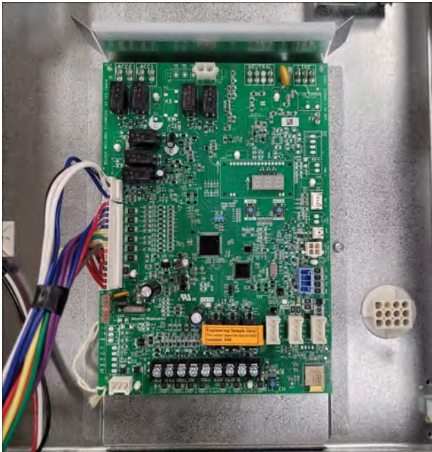
Figure 38. Control harness and inducer communication harness
