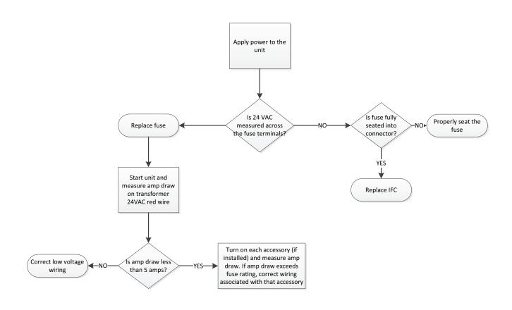
Continuous FAN on this unit is limited to TAP 1 only. No field adjustment can be made. If troubleshooting other speed taps, use the method as outlined below using the voltages listed for the tap number being used
