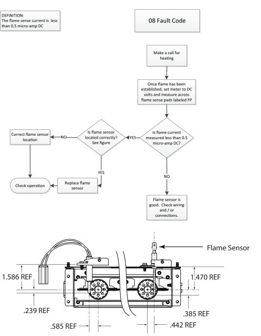
There are two flame sense pads located on the IFC, marked "FP". To measure flame current, use a VOM set to DC volts. Flame current will vary depending on the type of meter used. Typical flame current ranges from 0.75 – 3.0 micro-amps (0.75 – 3.0 VDC)
