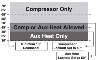
AN OUTDOOR TEMPERATURE SENSOR MUST BE ENABLED FOR LOCKOUT SETTINGS TO BE AVAILABLE. Lockout options are located in the Installer Setup>Lockout Settings.
