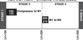
Note: Stage Thresholds do not apply to Variable Speed Outdoor Unit operation.
