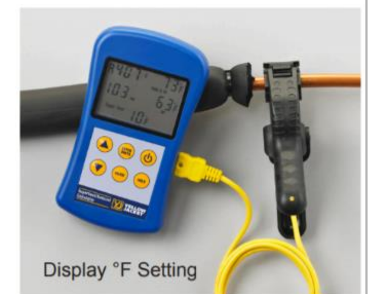
Display °F Setting SuperHeat/SubCool measurements simplified, especially when converting systems to use some of the newer refrigerants
